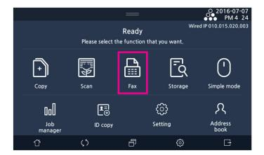
Place a document on flatbed glass or automatic reverse document feeder (ARDF). When sending a fax from flatbed glass, make sure there is no document on ARDF.
