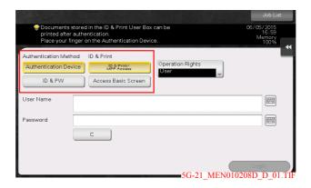
Check that [ID & Print/MFP Access] is selected in [ID & Print], and place your finger, IC card, or NFC-compatible Android terminal on the Authentication Unit.
