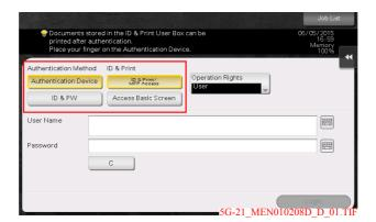
Check that [ID & Print/MFP Access] is selected in [ID & Print], and place your finger, IC card, or NFC-compatible Android terminal on the Authentication Unit.
